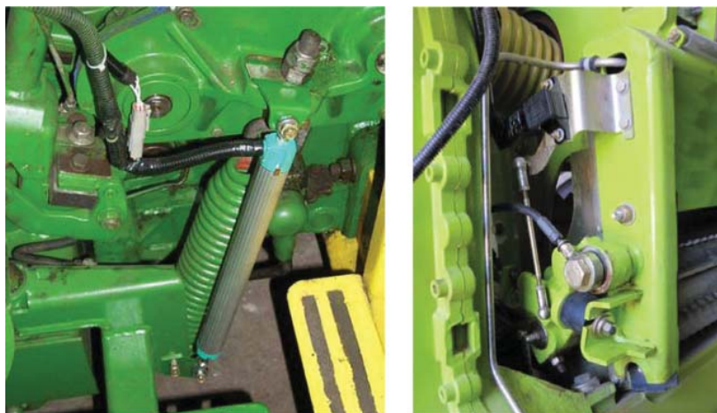
Figure 2. Linear (right) and angle (left) sensor for measuring feed roll movement (Digman and Shinnars, 2013).
