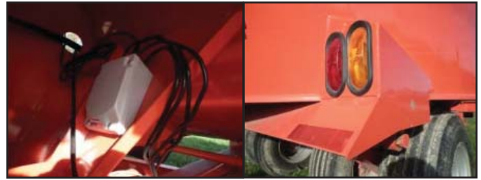
Figure 3. Junction box (left) tail lights and reflector (right).
