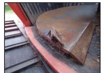
Figure 2. Vertical mixer auger scraper bar and kicker.
