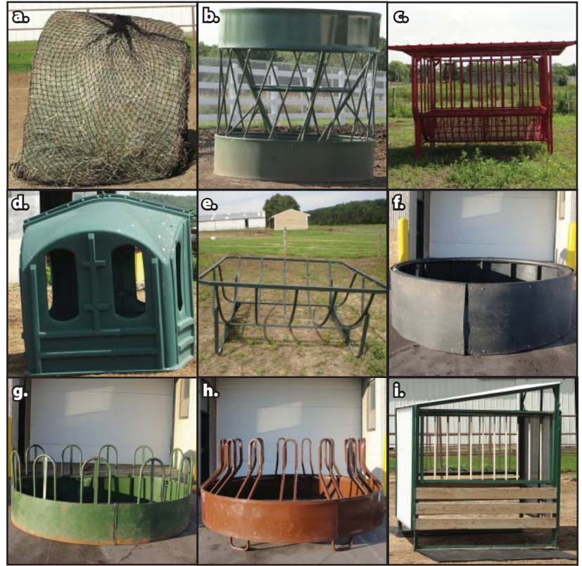
Figure. Round-bale feeder designs: a. Cinch Net, b. Cone, c. Covered Cradle, d. Hayhut, e. Hay Sleigh, f. Ring, g. Tombstone, h. Tombstone Saver, and i. Waste Less
