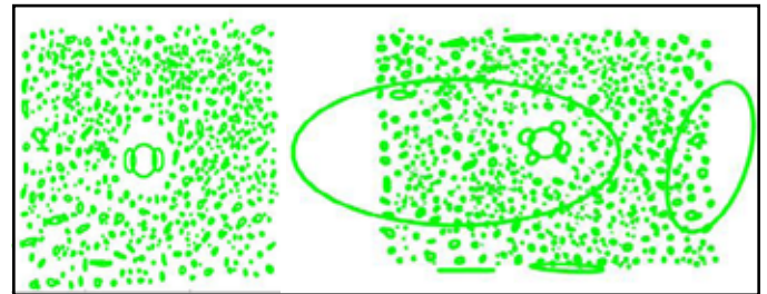
Figure 1. Image analysis results of kernel processing score. Good image analysis results from the app (left) show many individual particles; bad image analysis results from the app (right) show large circles caused by glare in the image.
