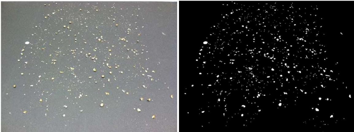
**Figure 2. Original image of sample 100 taken with the smart phone (8 Megapixel resolution) (left). Black and white processed image of sample 100 taken with the smart phone (right).**
