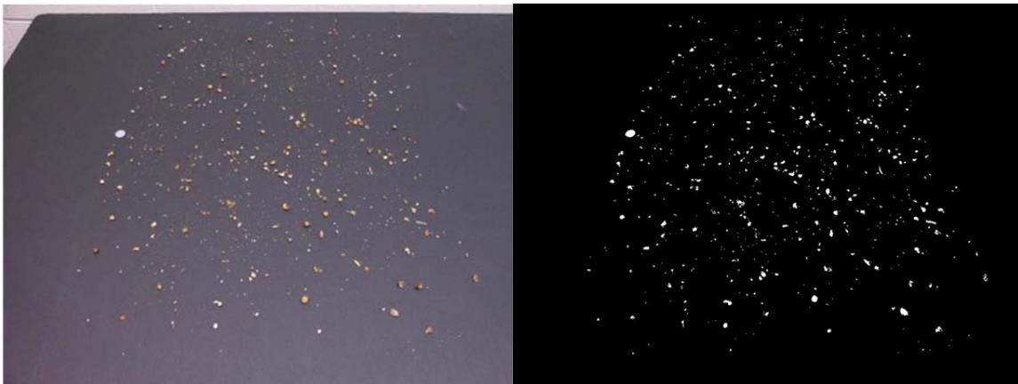
**Figure 4. Original image of sample 100 taken with the Nikon S6100 (16 Megapixel resolution) (left). Black and white processed image of sample 100 taken with the Nikon S6100 (right).**
