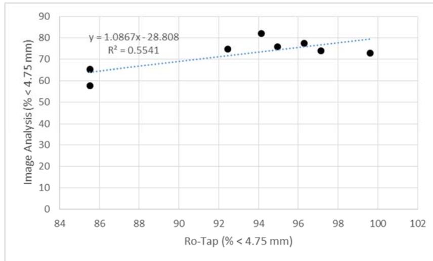
**Figure 8. Linear regression results comparing the percent of the sample smaller than 4.75 mm determined via image analysis and traditional Ro-Tap methods.**
