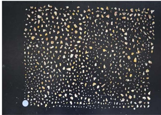
**Figure 1. Original image format for image based particle size distribution analysis. Layout dimensions of approximately 31 x 31 cm and a United States Penny located in the lower left corner for scaling purposes.**
